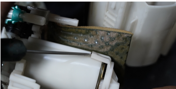
6.Disconnect the fuel pump from the pump assembly and disconnect the electrical wire.
